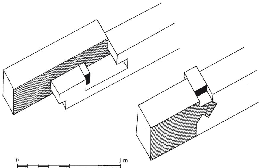
Fig. 13. Assembly of beams in a horizontal plane (line of Jupiter). The elements indicated in black represent the keystones, ensuring consistency.
