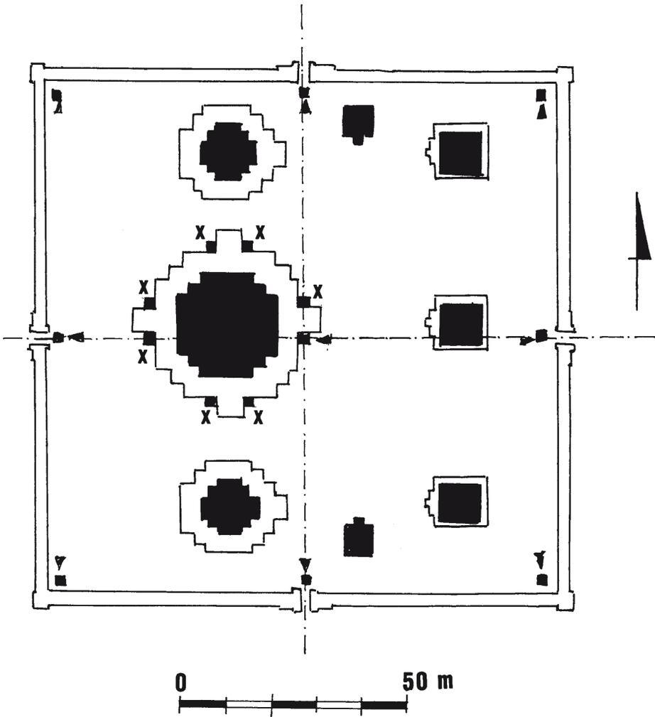
Fig. 9. Prambanan, schematic plan of the upper terrace and layout of the temples housing the bench-marks. The letter X indicates the base temples and the arrows point out the location of the doors.
