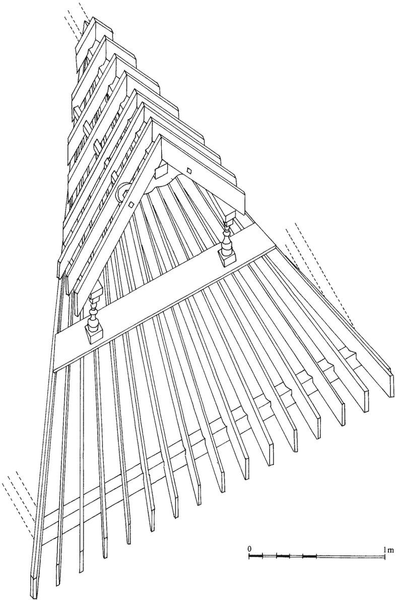
Fig. 25. Implementation of the frame of a false gable over a building covered with a radiating frame (Battambang region).
