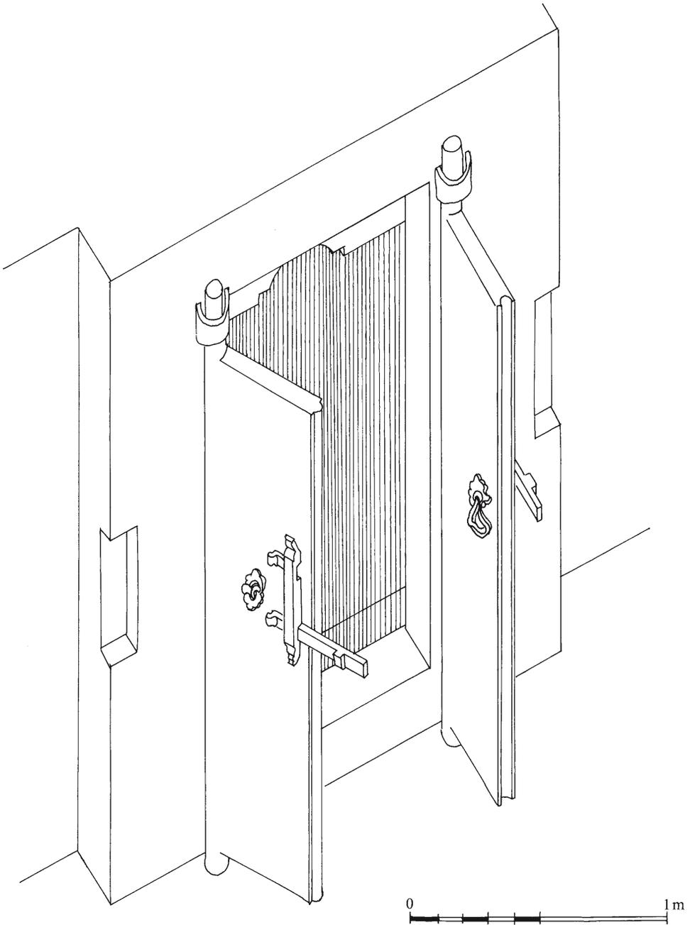
Fig. 50. Ceylon, interior view of a door of the palace of Kandy and its setting in the masonry. A complete door, similar but with a wooden door frame, is on display at the museum of Kandy.
