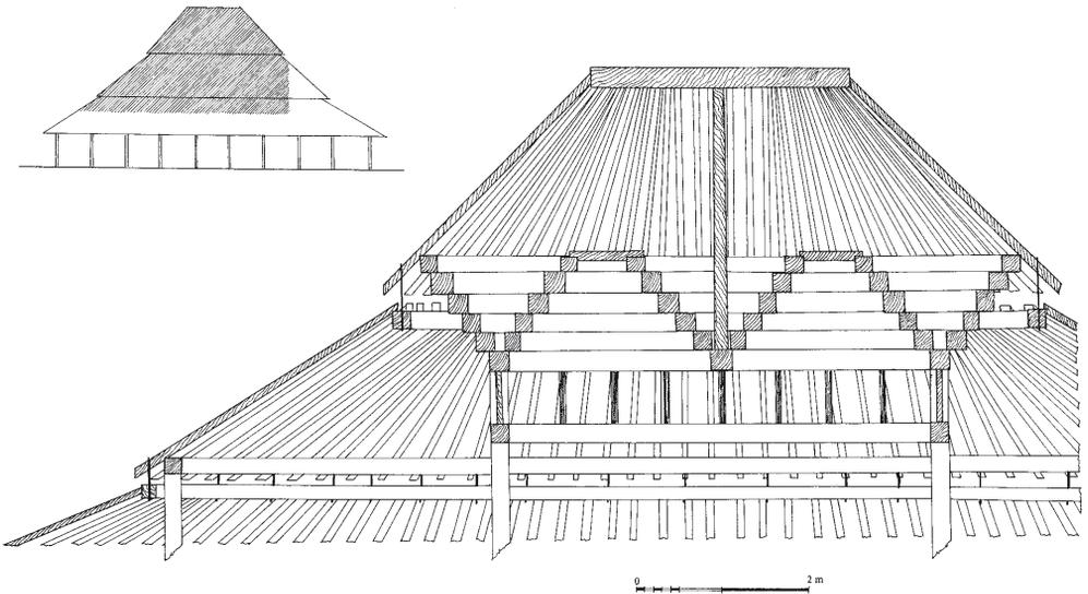
Fig. 31. Radiating frame of a pendopo in Solo, Java.
