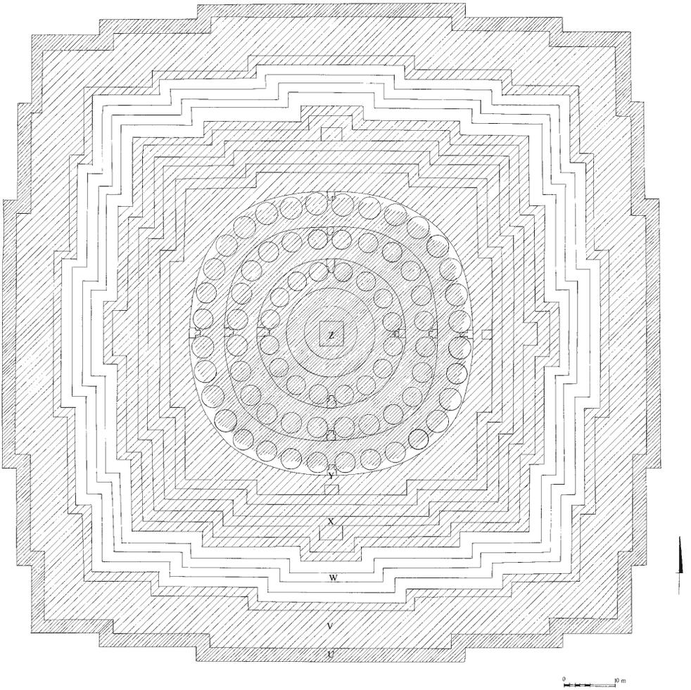
Fig. 5. Borobudur, plan of the entire group of successive layouts. W, first layout; X, second; Y, third; Z, fourth; V and U, fifth.
