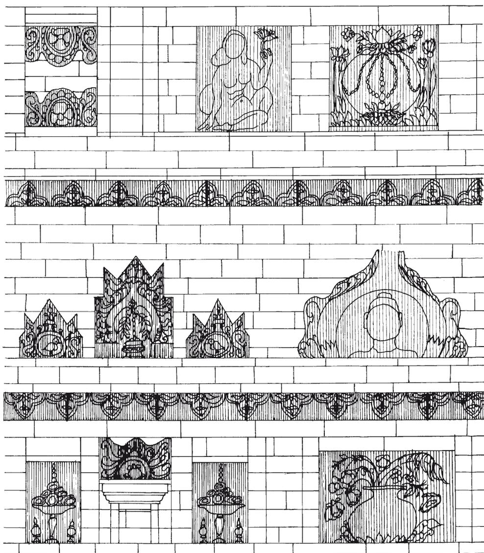
Fig. 89. Candi Gunung Gangsir, Java, detail of décor set into the brick bond of the base of the sanctuary wall; the different elements modelled into the terra cotta are hatched.
