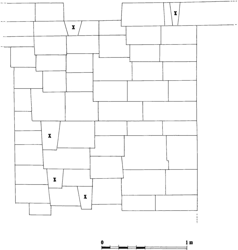
Fig. 85. Bayon, eastern wall of the first gallery, south side, stereotomy detail. The stones marked "X" are striking wedges.
