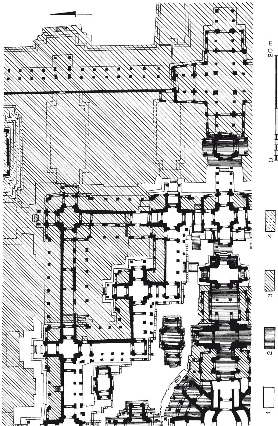
Fig. 97. Bayon, partial plan of north-eastern quarter, showing the four construction steps (marked 1, 2, 3 and 4). The structures indicated by dotted lines represent the galleries constructed after the third step and destroyed before the last step.
