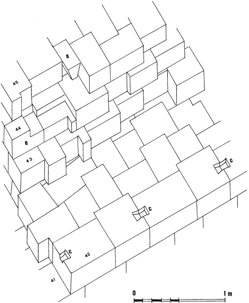
Fig. 80. Borobudur, courses 41 and 45 of the internal base of the first gallery, implementation of double dovetail spikes, C, of the representation (based on pl. LII of *L'Histoire architecturale du Borobudur*, op. cit.).
