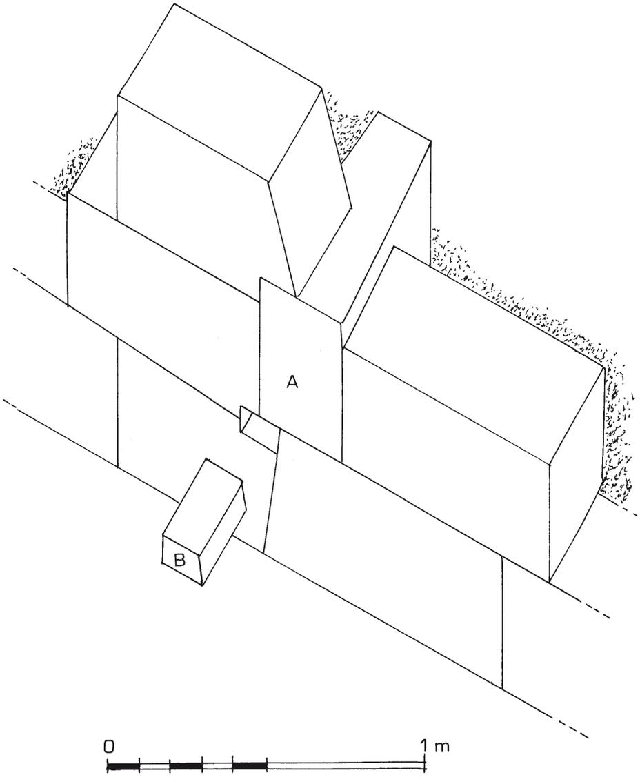
Fig. 78. Stereotomy of the base of the foundation of a building in Mihintale (Ceylon). A, striking wedge in the horizontal plane; B, wedge put into place after the course was adjusted.
