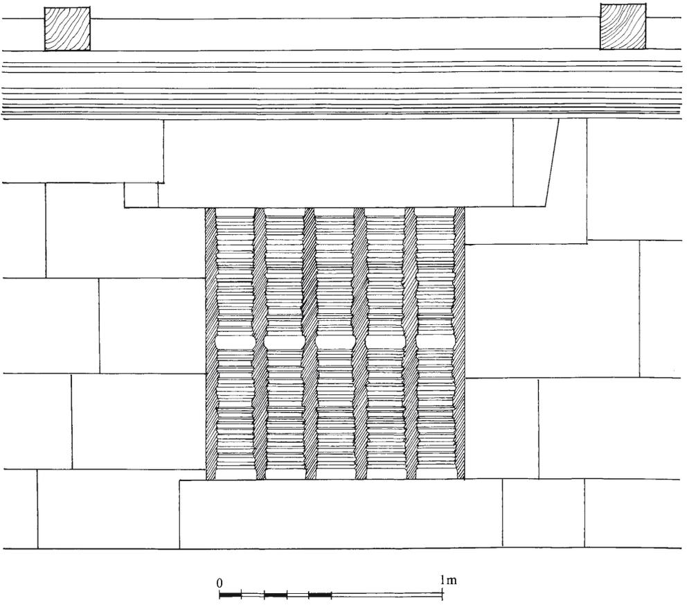
Fig. 42. Sandstone window of room N of Preah Vihear, inner side.
