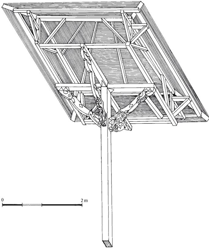
Fig. 30. Radiating frame over a central pillar in Java.
