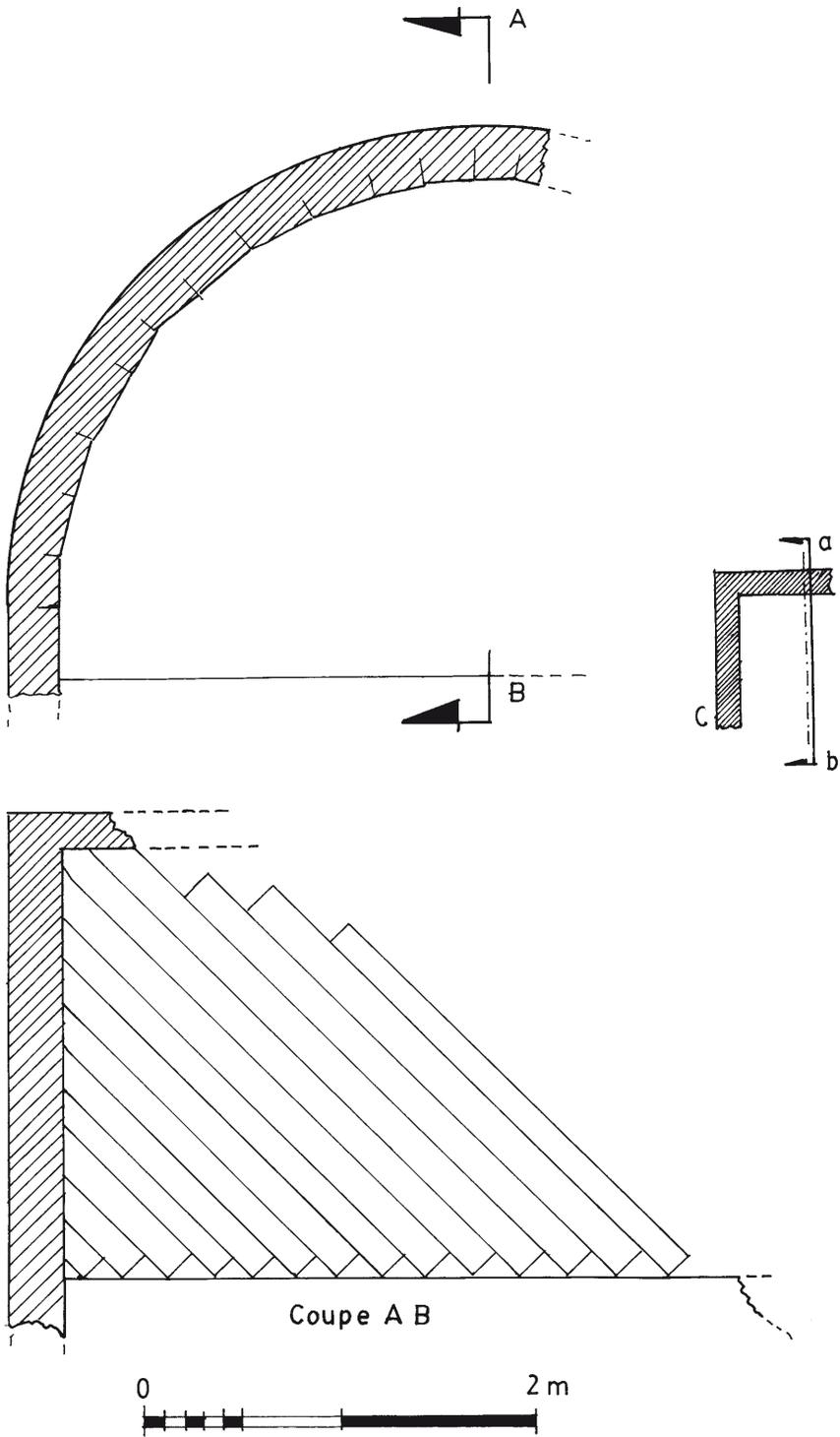
Fig. 56. Barrel vault constructed with unburnt bricks.
