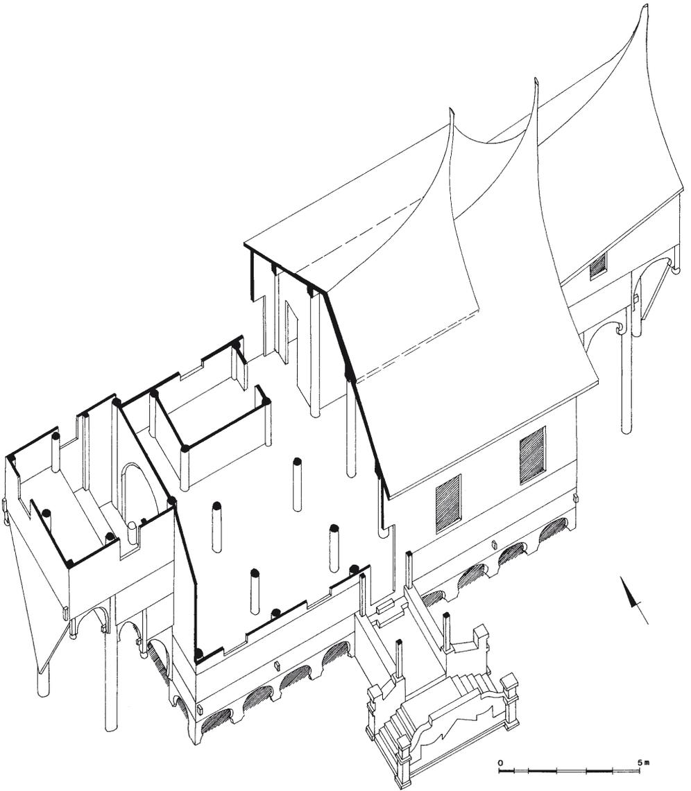
Fig. 39. Minangkabau house, axonometry, Sumatra, Indonesia.
