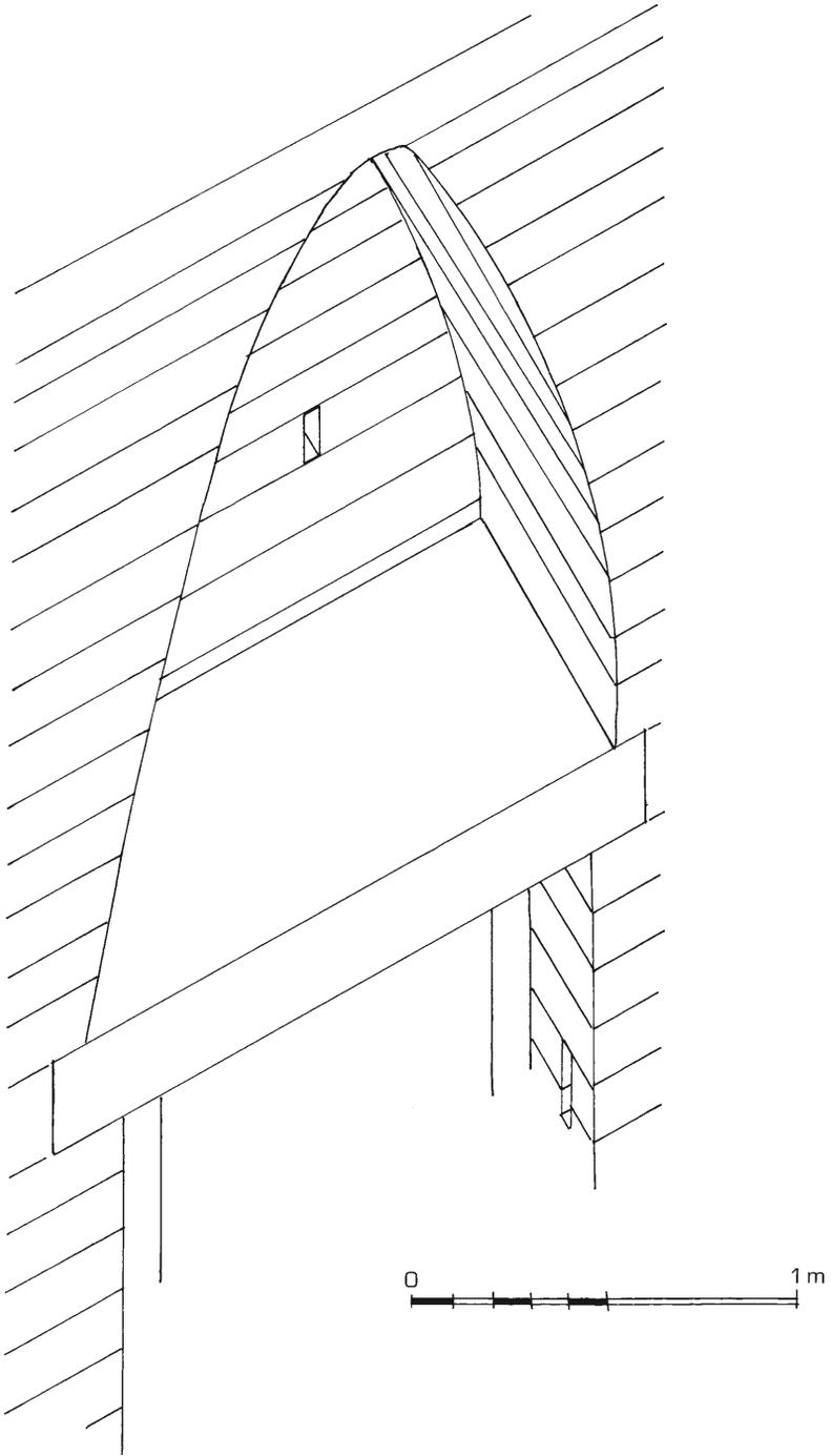
Fig. 79. Discharge arch above the lintel of a door at Candi Bhima in Dieng, Java.
