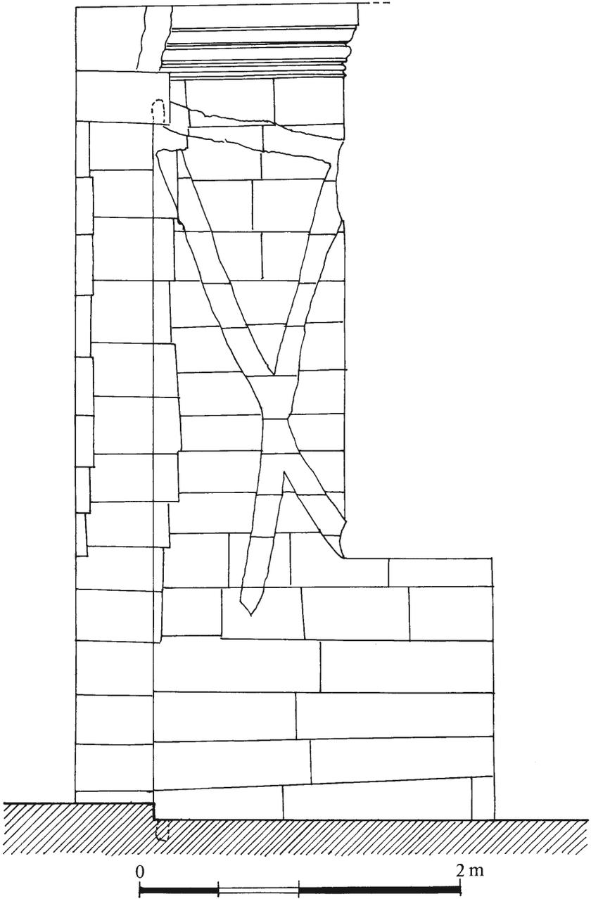
Fig. 53. Angkor, temple of Ta Prohm, jamb of the northern door showing the casement of the repaired leaf.
