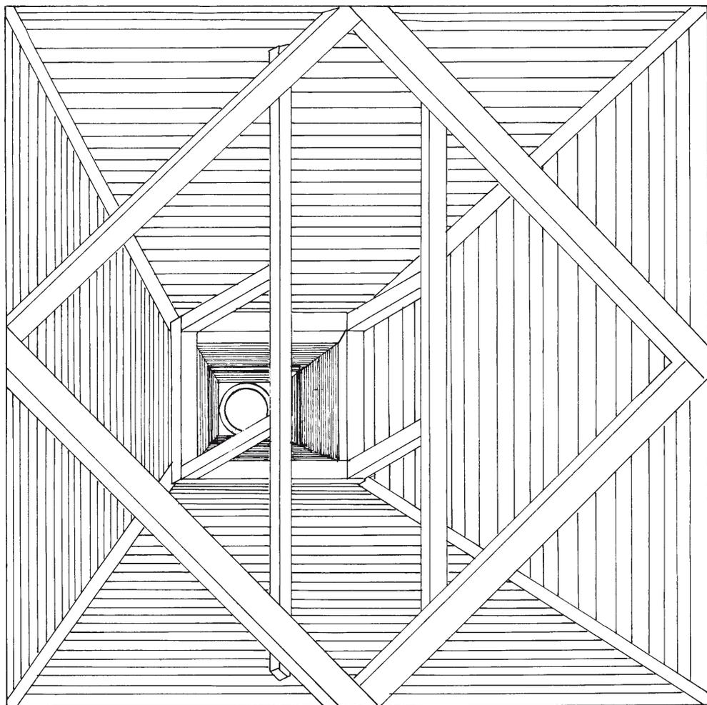
Fig. 22. Bending frame on a square plane, panelled (pavilion of the lacquer Buddha at Salé, Burma).
