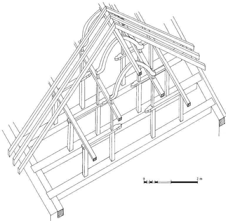
Fig. 27. Bending frame without crown post in the Darasuram region, India.
