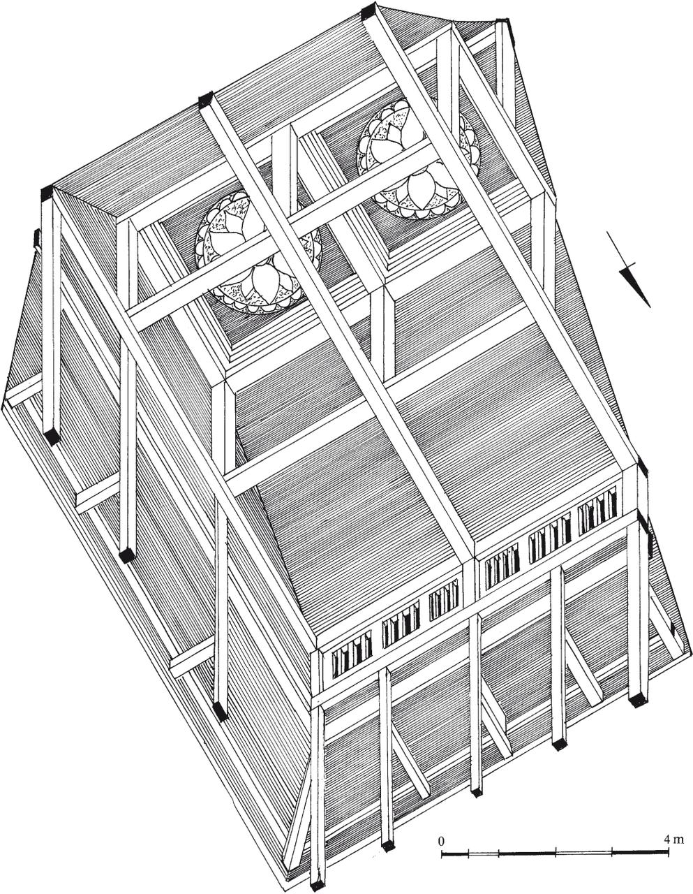
Fig. 23. Bending frame with partial ceiling and panelling, in Amarapura, Burma.
