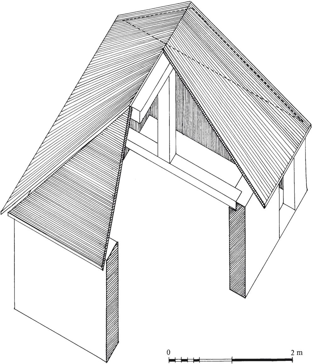
Fig. 33. Axonometry of a roof with four sloping sides resting on a frame cut down to three pieces: a tie-beam, a crown post and a ridgecap (Bali).
