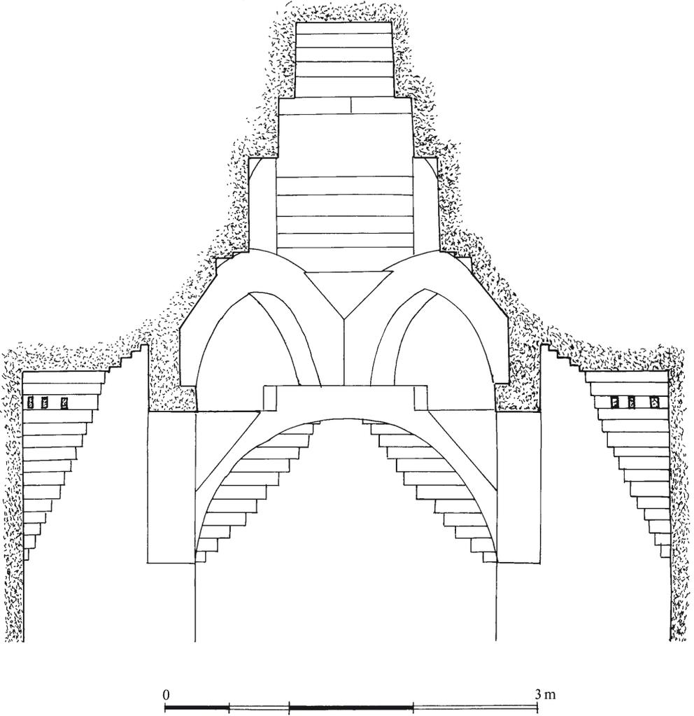
Fig. 60. Darasuram, temple of Amman, cross section of the cella ceiling.
