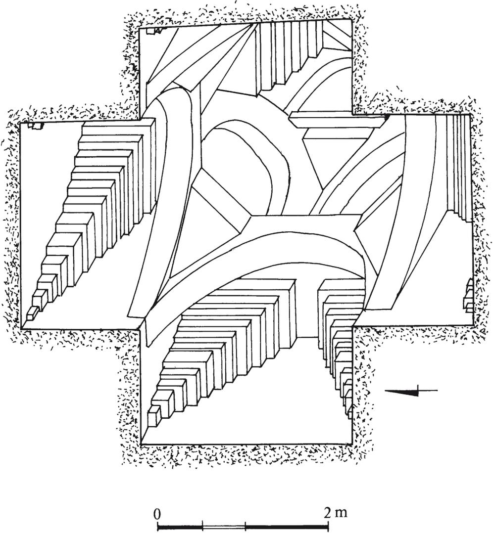
Fig. 61. Darasuram, axonometry of the intrados of the vault of the Amman temple cella.
