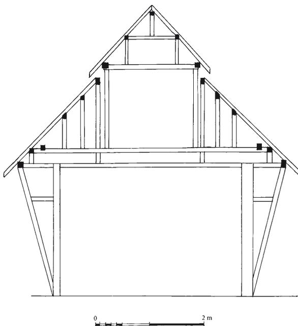
Fig. 26. Fragment of a bending frame with two sides over a structure with warped walls at Luang Prabang in Laos.
