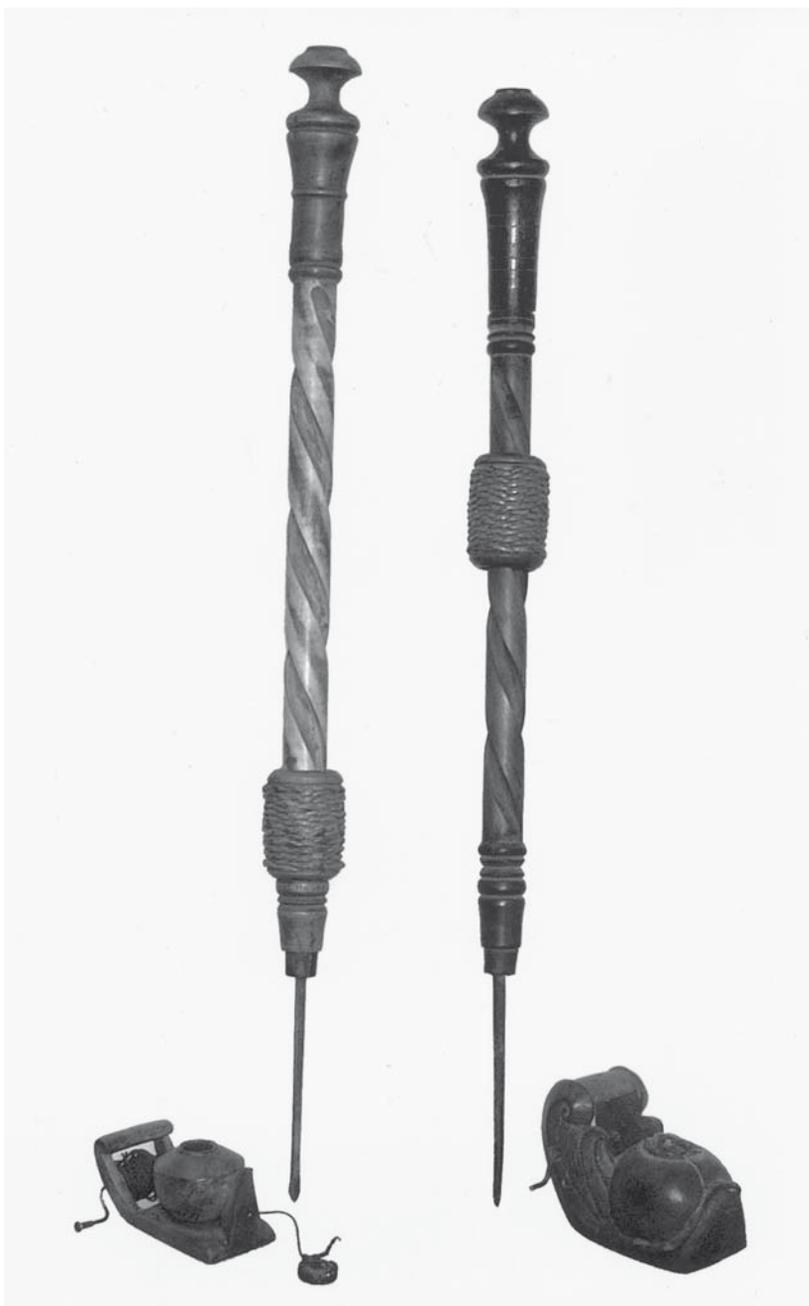
Ph. 6. Indonesia, Java and Sumatra. Archimedes drills (standing tools) and *riolet* wheels on the bottom.
