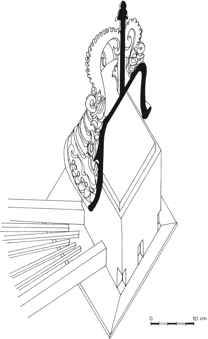
Fig. 72. Bali, implementation of a ridge finial over a radiating frame.
