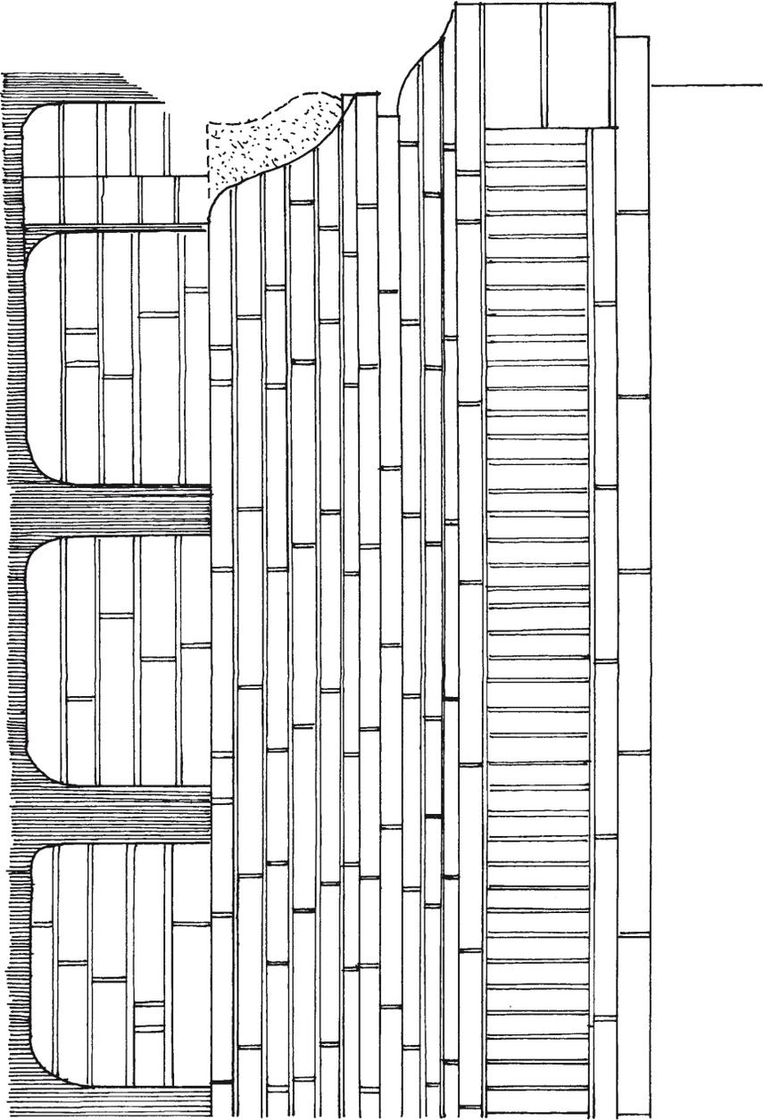
Fig. 63. Mingalazedi, masonry detail of the capping of the first floor, western façade.
