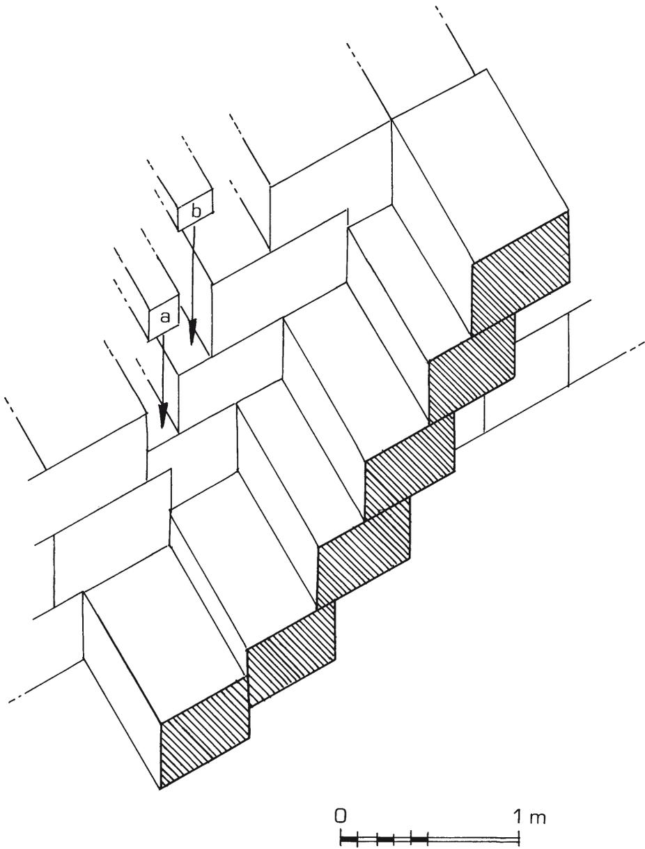
Fig. 86. Darasuram, stereotomy of the northern staircase of the entry pavilion II/east, stones a and b are wedged.
