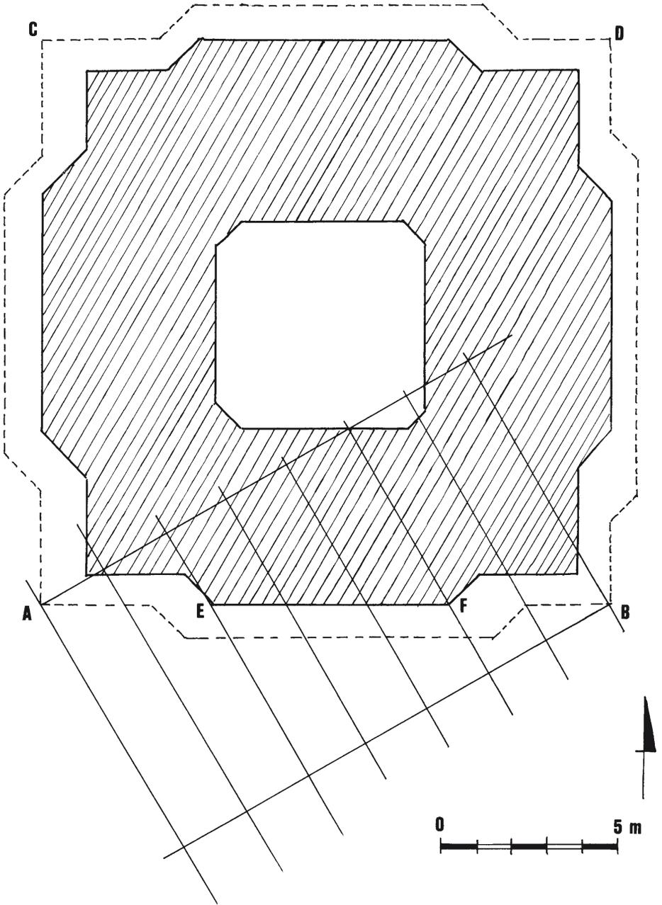
Fig. 8. Gangaikondacholapuram, layout of an octagonal false floor of the central tower.
