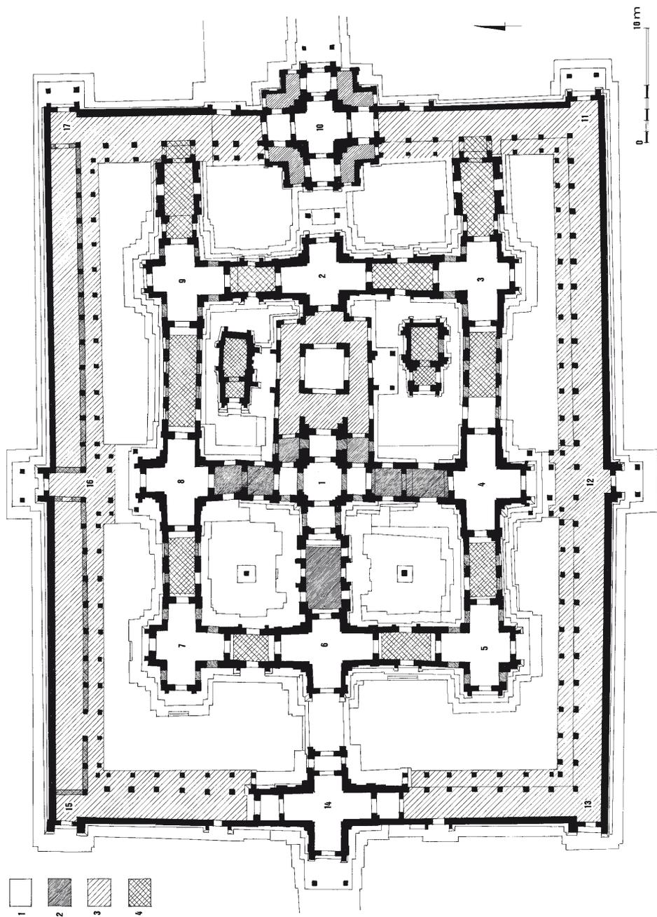
Fig. 95. Bantay Kdei, Cambodia, plan of different construction steps of the temple.
