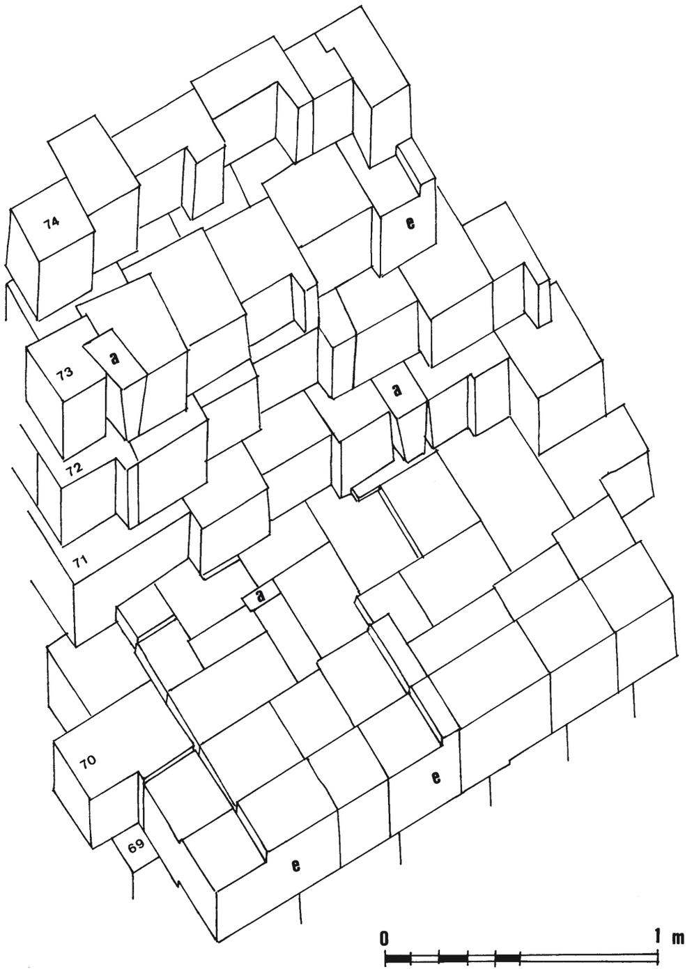
Fig. 81. Borobudur, stereotomy of the internal base on the level of the third gallery of the 69<sup>th</sup> to the 74<sup>th</sup> course, with striking wedge, and angle bar in the vertical plane (based on pl. LIII of *L'Histoire architecturale du Borobudur*, op. cit.).
