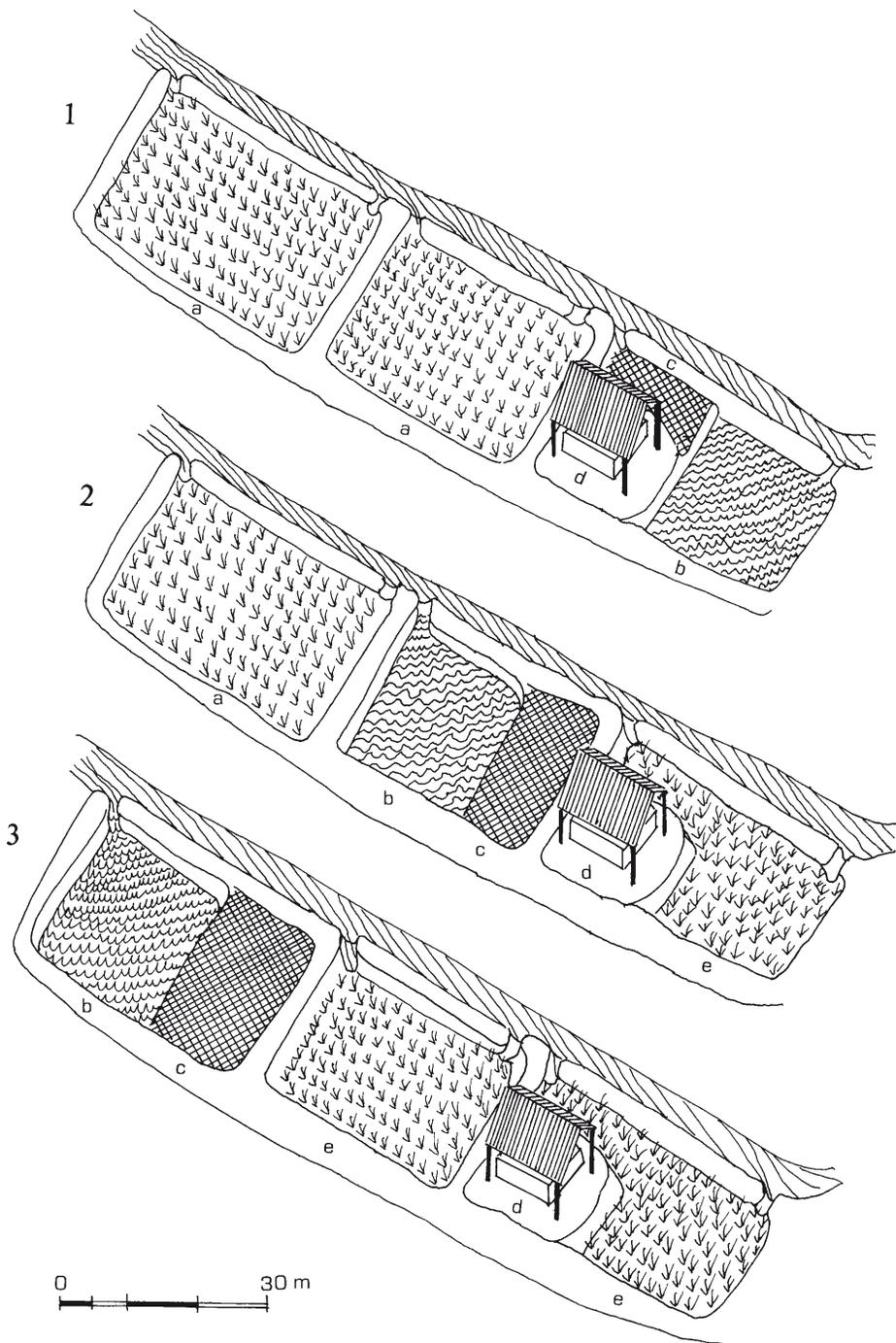
Fig. 58. Creation of bricks in Sawanti (village near Magelang, Java, 1977-1978) at the period of the drop in the rice paddy water levels. Legend: a, rice paddies at normal level before work; b, area where the paste is prepared; c, brick drying area; d, oven; e, rice paddies at normal level after the work.
