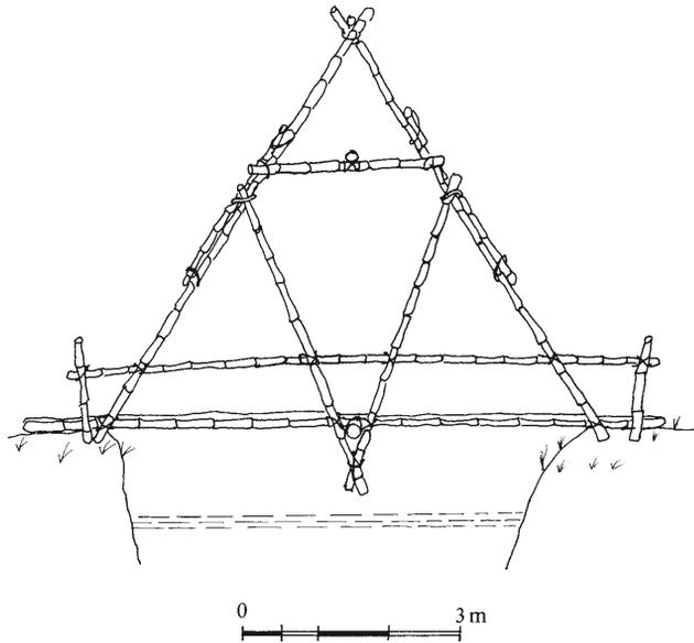
Fig. 40. Bamboo bridge over the river Kanta, Siem Reap region.
