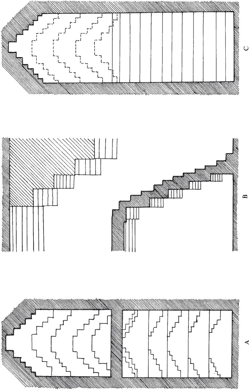
Fig. 64. Pagan, restitution of the string and roofing of a staircase, based on structure No. 2182 from the inventory taken by Pierre Pichard, *op. cit.*, vol. VIII.
